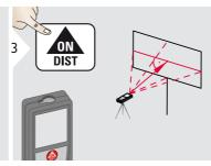
Aim perpendicular to the horizontal center line of the area. This area must be perfectly flat on the vertical plane.
